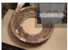
The final project of the DVD is a ribbon bowl—a structure that curves back upon itself in a way that could never be turned directly. Tibbetts begins with concentric segmented rings, then builds up a structure rather like a truck wheel and hub, which he turns to final shape. He then cuts the turning into pieces, which he rotates and assembles into his final concept.
